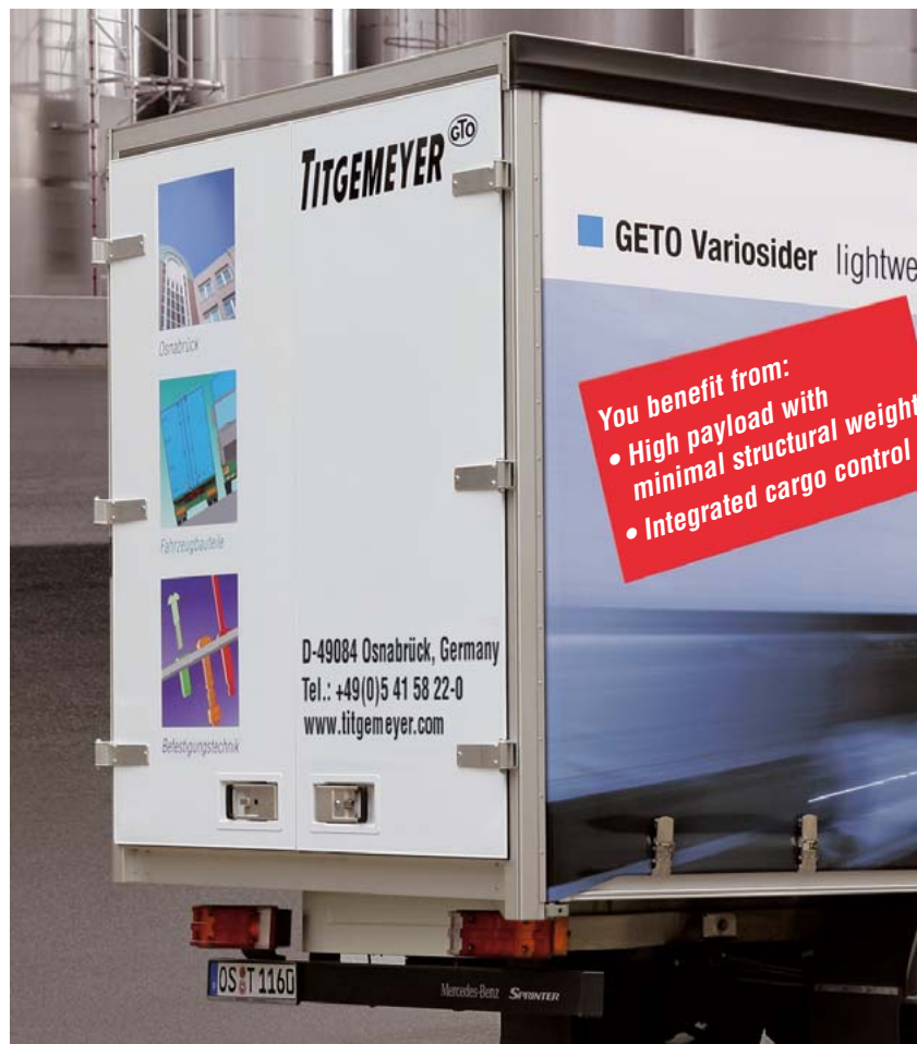
GETO® Variosider with double-leaf rear doors and recessed locks
