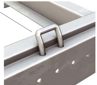
Cargo control Integrated lashing rings for securing of loads
